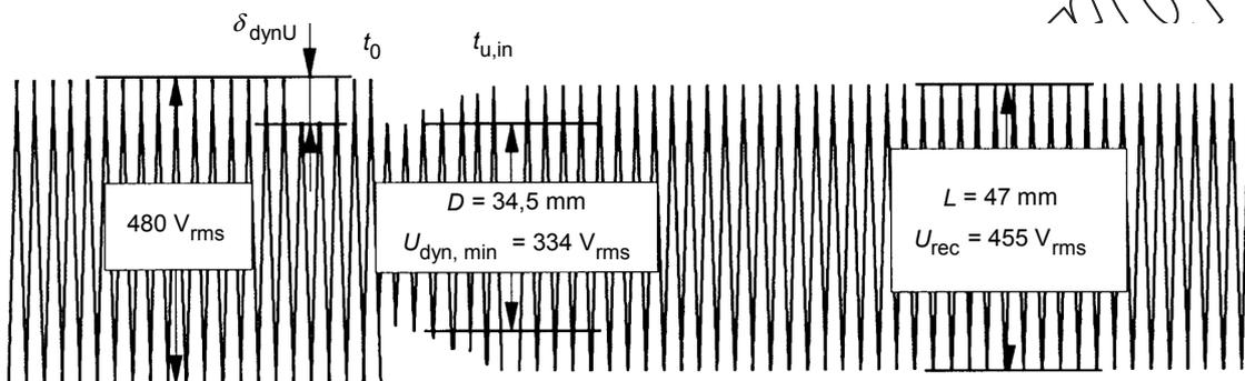
Oscillogram of terminal voltage
