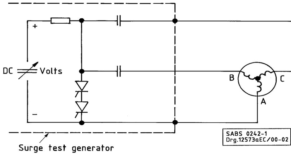
Figure 4 — Surge comparison test set up comparing phase B with C
