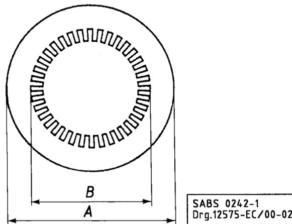
**Figure 8 — Dimensions for calculation of core area**
