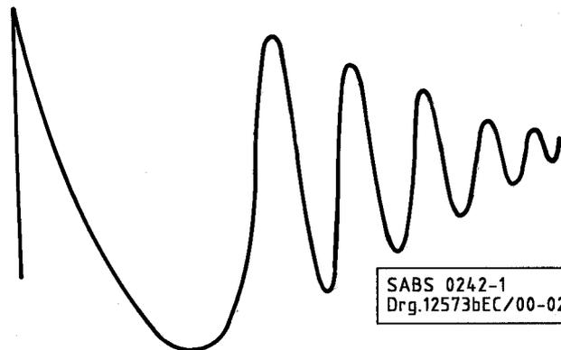
Figure 5 — Typical surge waveform of two phase windings without shorts between turns
