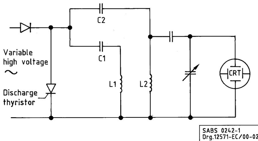
Figure 2 — Typical surge comparison test circuit
