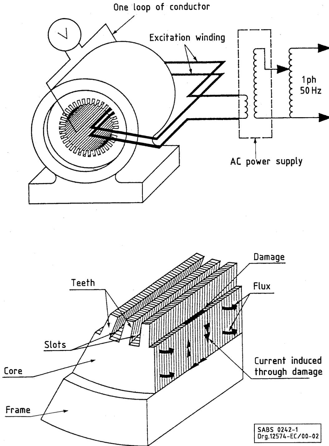
Figure 7 — Schematic diagram of a typical test circuit for a core test
